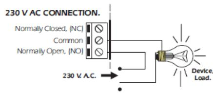
**ABOUT THE OUTPUT:** During operation of the circuit, and according to its load, may cause a fluctuation or an incorrect operation of the output. If this happens, install an anti-spark circuit, (V. 100nF/400 capacitor and resistor 47. ½ W), between the two relay contacts used in the connection.
