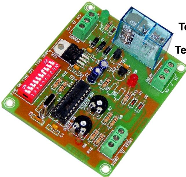
**Digital timer with 2 adjustable times with potentiometers**
